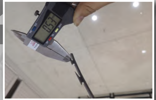
Barb Thickness Test
